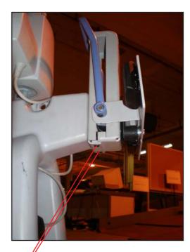
Remove four screws to access the kneepad height adjustment mechanism.
