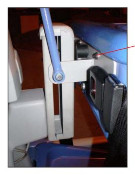
Remove screws securing kneepad to support plate
